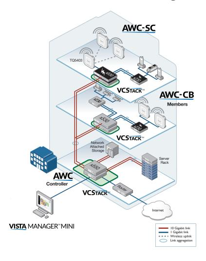
Allied Telesis Autonomous Wave Controller (AWC) offers solutions for two of the most common problems with Wireless LANs: initial setup complexity and on-going performance degradation. Initial WLAN set-up usually requires a site survey to achieve the best coverage; and performance of WLANs can often change over time as external sources of radio interference reduce coverage and bandwidth. These issues can be time-consuming to identify and resolve.
