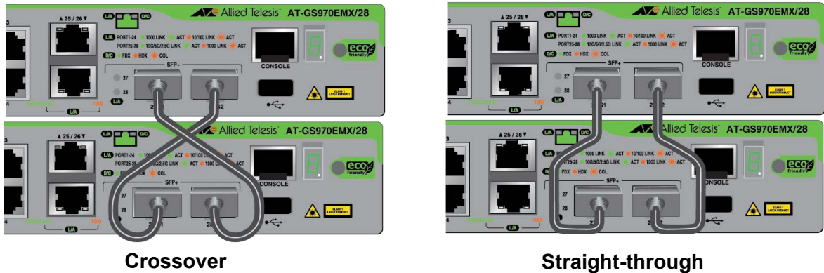
Figure 12. Stack Trunks of SFP+ Ports S1 and S2 for Two Switches
